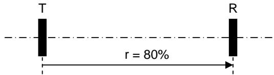
Note that, independently of the orientation of the buried transmitter, the searching person can always orient the receiver such that the antenna coil windings will be perpendicular to the field lines. Thus, the parallel orientation represents the worst of the cases that can always be achieved.
