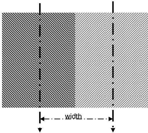
The wider the search strips, the more area can be covered within a given time span. However, widening the search strip also increases the probability that a buried victim is not detected. Since the actual range of a beacon is always dependent on the relative orientation of the transmit and receive antennas, there is no guaranteed minimum range.
