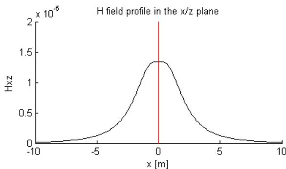
Fig. 7 horizontal dipole
