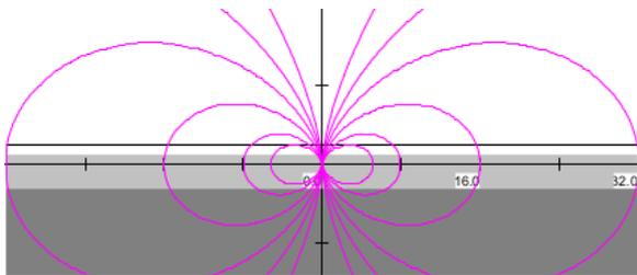
Fig. 10 vertical dipole
