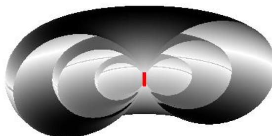
Fig. 2 vertical dipole
