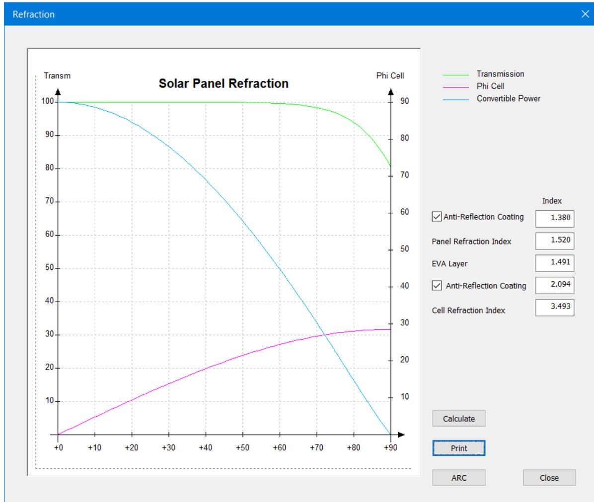
This dialog serves to specify and evaluate the effects of the various layers of a solar panel above the actual energy conversion medium, i.e. the bulk silicon or the heat absorber.
