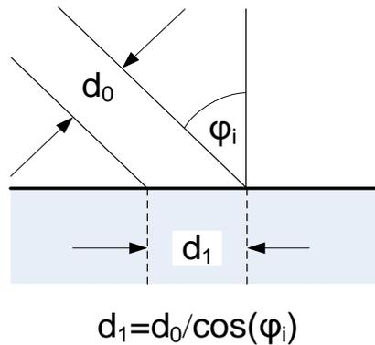
The yield of solar panels is specified assuming that the incident radiation is normal to the surface of the panel. So the incident radiation must be multiplied by  $\cos(\varphi_i)$  for obtaining the radiation that is normal to the surface of the panel.
