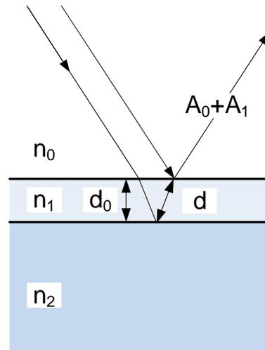
The thickness of the ARC layer is chosen so that the group delay of  $A_1$ , the refracted and reflected radiation amplitude at the exit to the top medium, is equal to half the period of the incident light. So the reflected components  $A_0$  and  $A_1$  (almost) cancel each other, and a larger portion of the incident power is propagated into the layer underneath the ARC. The optimum index of refraction for the ARC material is
