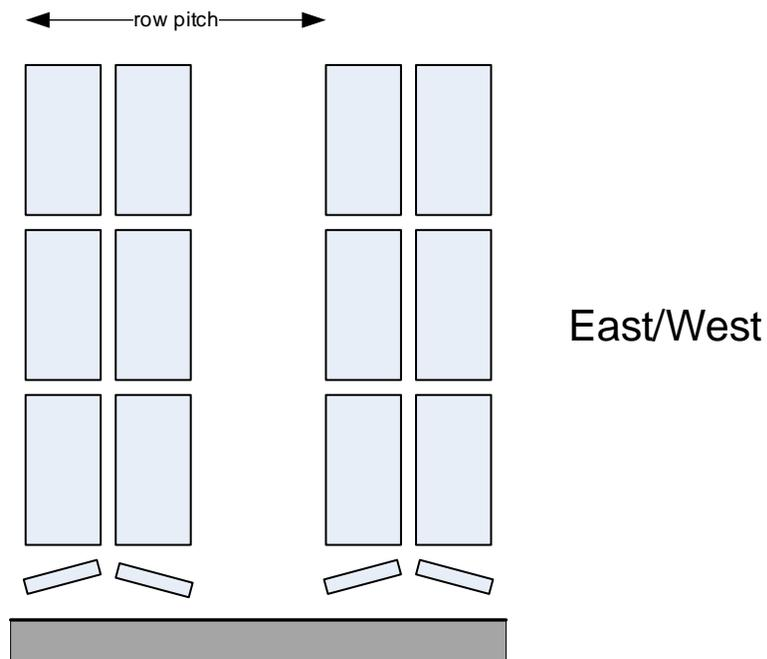
In this configuration, half of the panel rows are facing East, and the other half of the rows are facing West. Again, the orientation may be quite different depending on the roof orientation.
