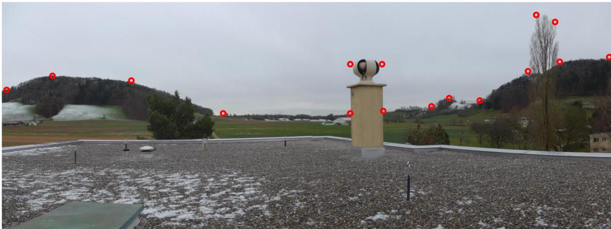
A file may be provided with a list of vertices of the horizon line for a specific location. With this data, the shading of solar panels by the horizon can be taken into account.
